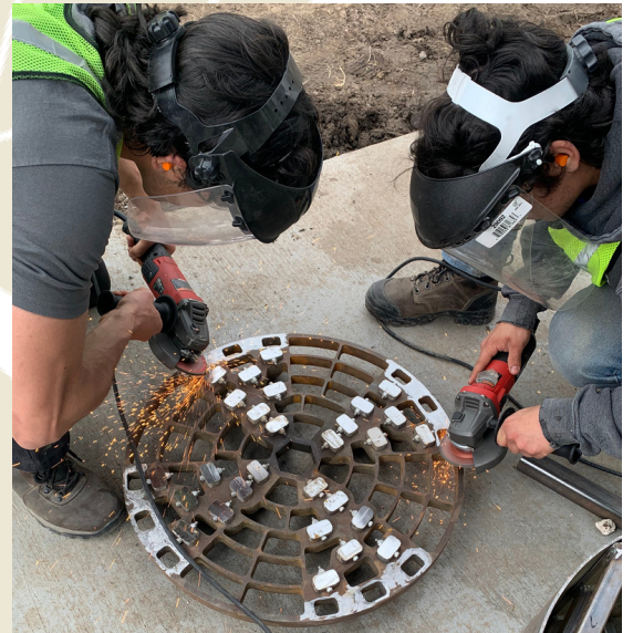
Mateo and Ben grinding the cutting wheel after learning our outer cutting teeth would not arrive in time
